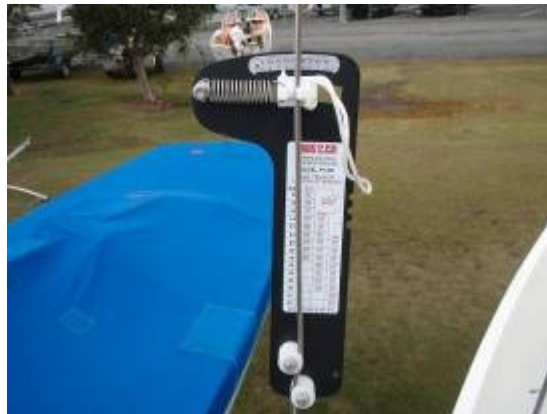
Set the BASE cap tension at #18 (PT-2)
